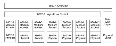
This family of International Standards deals with the Physical and Data Link layers as defined by the ISO/ IEC Open Systems Interconnection (OSI) Basic Reference Model (ISO/IEC 7498-1 : 1994). The access standards define seven types of medium access technologies and associated physical media, each appropriate for particular applications or system objectives. Other types are under investigation.
