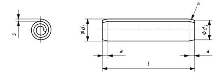
a Swaged chamfer at both ends.
