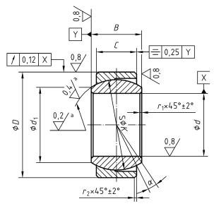
a 0,4 for spherical surface with dry-film lubricant; 0,2 for non-coated surface
