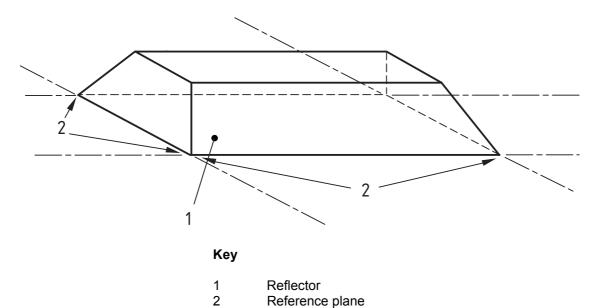
Figure 1 — Radiation reference plane
