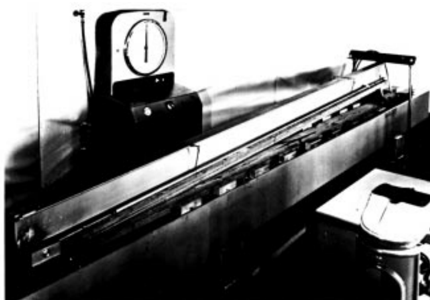
FIG. 7 Compression of Long Slender Structural Member
