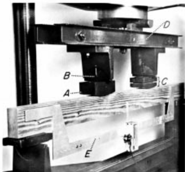
FIG. 4 Example of Curved Loading Block, A, Load-Alignment Rocker, B, Roller-Curved Loading Block, C, Load Evener, D, and Deflection-Measuring Apparatus, E
