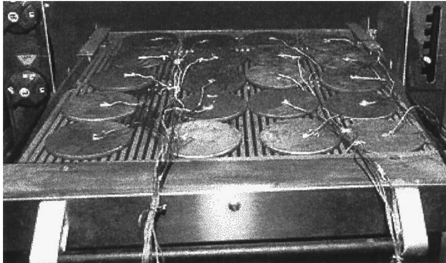
FIG. 2 Thermocouple Disk Placement
