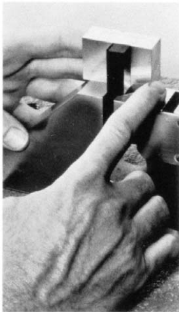
FIG. 4 Jig for Positioning Specimen for Clamping
