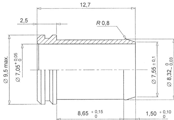
Figure 1 — Sleeve without sealing
