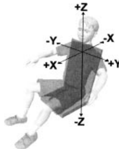
FIG. 1 Patron Containment Area Acceleration Coordinate Axes
