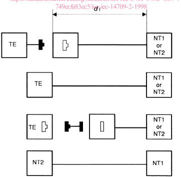
$d_1$  is the distance between the NT1 and the point of connection of the customer's terminal equipment.  $d_1$  also applies to the distance between NT1 and NT2.
