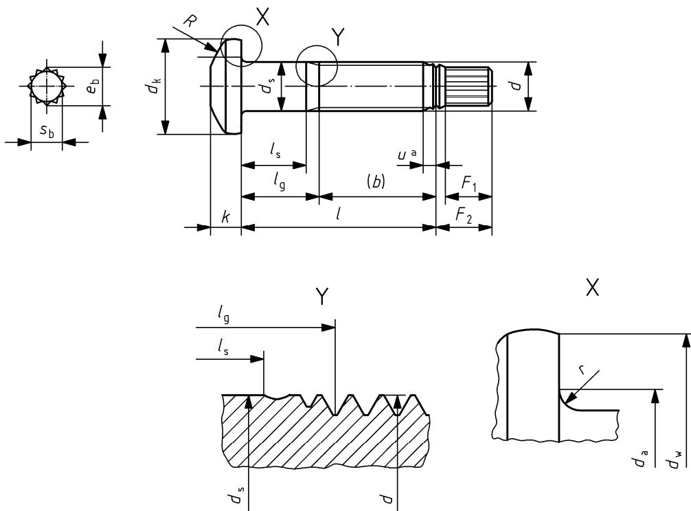
**Key****iTeh STANDARD PREVIEW****a** Incomplete thread  $u \leq 2P$ **(standards.iteh.ai)**NOTE The difference between  $l_g$  and  $l_s$  should not be less than  $1,5P$ .
