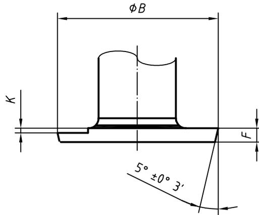
Figure 2 — Recess diameter plug gauge (gauge No. 2)
