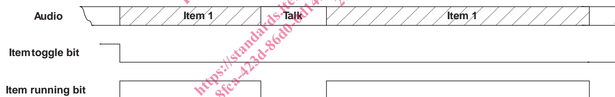
Figure 4: Setting of item toggle bit and item running bit when an announcer interrupts a programme item
