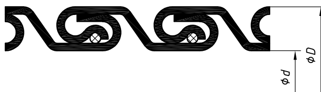
Figure 4 — Cross-section of a type DOP, double overlap, packed hose
