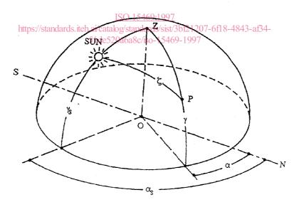
Figure 1 - Angles defining the position of the sun and a sky element P.
