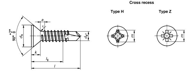
The function of the drilling point (diameter  $d_{\rm p}$ ) is specified in ISO 10666.
