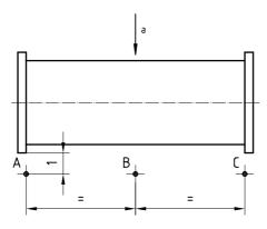
A, B and C are the measurement positions.
