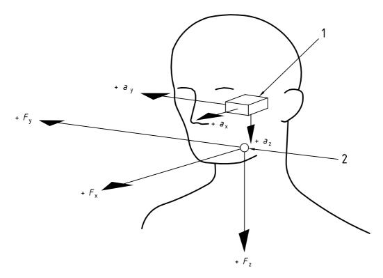
Triaxial accelerometer at centre of gravity of head Key
