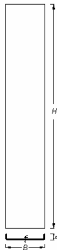
Figure 1 — Dimensions of a thermally toughened soda lime silicate channel shaped safety glass
