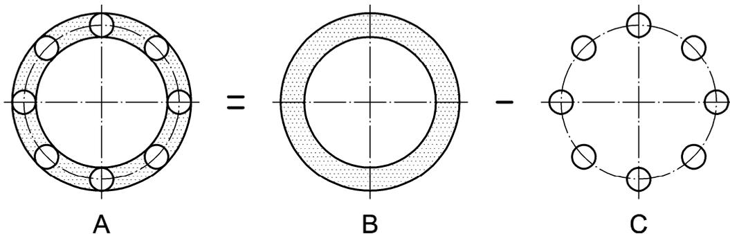
**Figure 7 — Gasket force calculation on bolt hole part**
