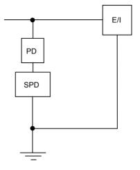
PD: protective device of the SPD SPD: surge protective device E/I: equipment or installation to be protected against overvoltages
