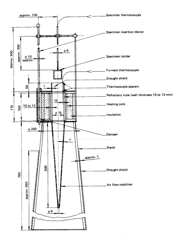
FIG. 1 - General arrangement : Non-combustibility apparatus
