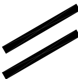
Figure 2 — Symbol for inclined joint
