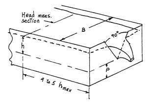
Limitations on geometry:<sup>B</sup>  $h/P \le 1.2$  $h/B \le 0.4$  $P \ge 0.3$  ft (0.1 m)  $B \ge 2$  ft (0.6 m) 0.15 ft (0.05 m)  $\le h \le 2$  ft (0.6 m)
