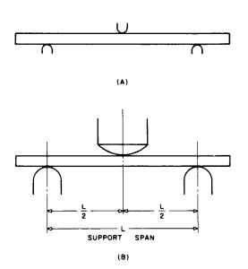
NOTE—(a) Minimum radius = 3.2 mm ( $\frac{1}{8} \text{ in.}$ ). (b) Maximum radius supports 1.6 times specimen depth; maximum radius loading nose = 4 times specimen depth.
