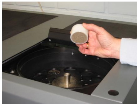
Figure 6 — Analysis of a dried and ground sample
