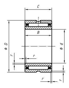
NOTE Needle roller bearings can be equipped with or without cage, with one row or two rows of needle roller and with or without lubrication groove and lubrication holes in the outer ring.
