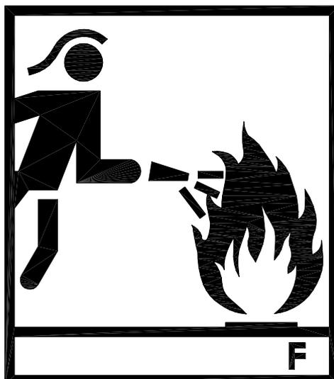
Figure 2 — Pictogram indicating protection against fire fighting hazards
