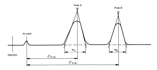
NOTE - The diagram shows an air peak, but this would not be seen with a flame ionization detector.
