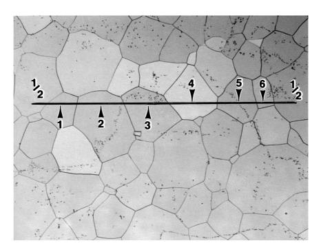
Interception, N, counts for a straight line on a single-phase grain structure where the arrows point to 6 intercepts and two line segments ending within grain (2 × 1/2 = 1 N) and N = 7
