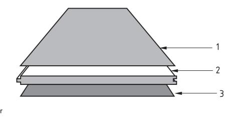
Key 1 Surface layer 2 Substrate 3 Backing
