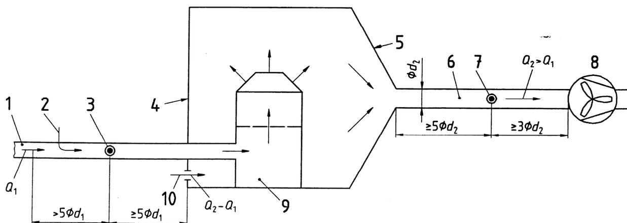
Figure 1 — Test rig with secondary air inlet
