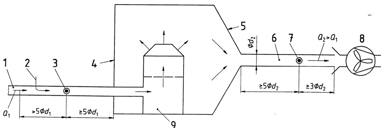
Figure 2 — Test rig without secondary air inlet
