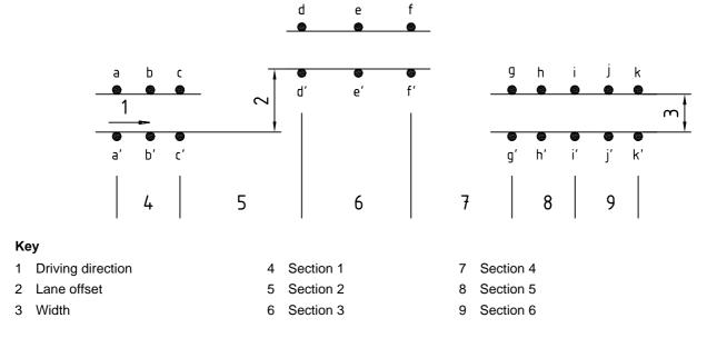
Figure 3 — Placing of cones for marking the double lane-change track
