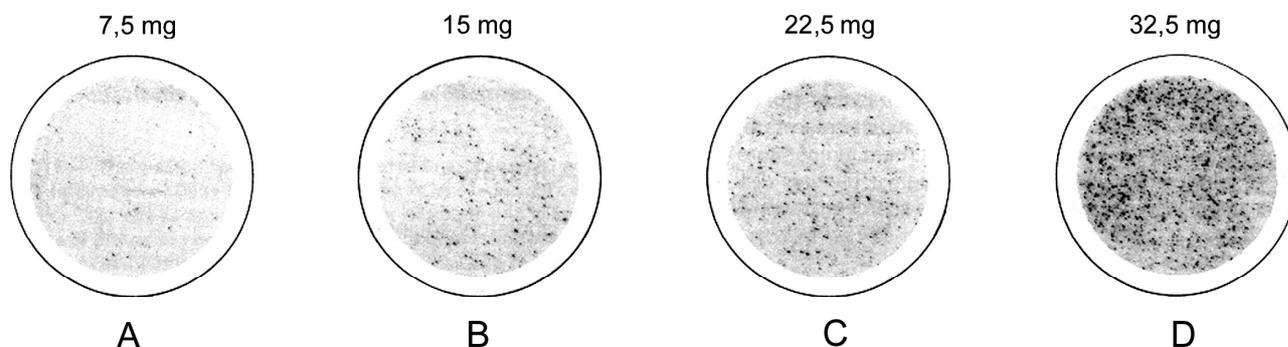
Figure 1 — Examples of standard scorched particle discs
