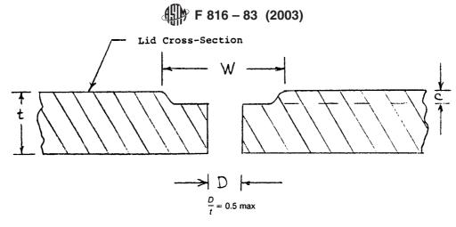
$D_{\text{max}} = 0.51 \text{ mm} (0.02 \text{ in.}), \text{ typically } 0.018 \pm 0.002 \text{ in.}$
