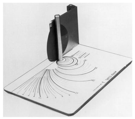
Arrange the clamp to hold the edge of the film on a line normal to the curves making up the measuring template. These curves may be computed as defined in 4.3. (standar) Type i
