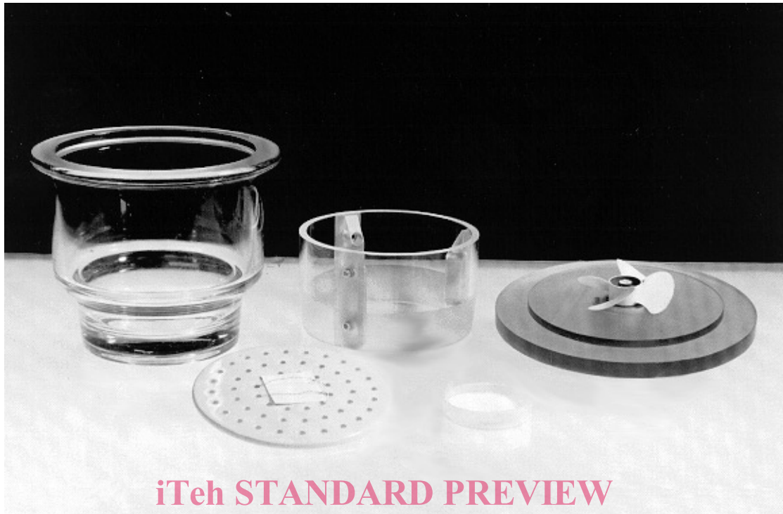
Figure 2 — Desiccator jar components
