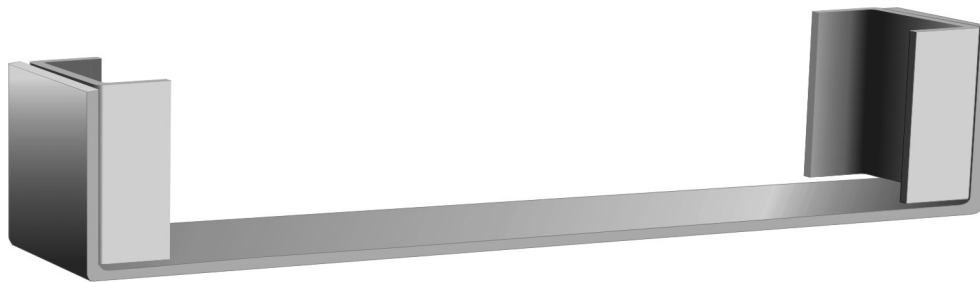
Figure 2 — Specimen jig to hold sandwiches
