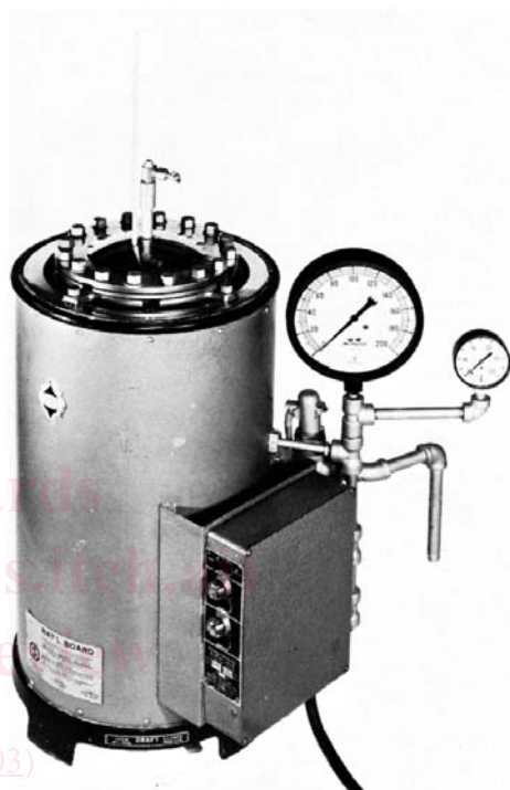
FIG. 1 Suitable Apparatus for Measuring Hydration Resistance of Basic Brick and Shapes (See 1)
