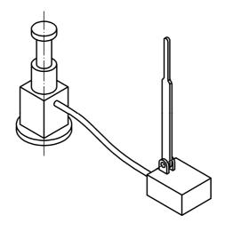
Figure 3 — Example of hydraulic jack without integrated pump
