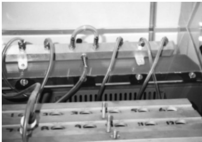
FIG. 7 Gassing Manifold for Venting
