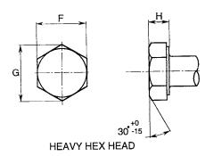
DIMENSIONS FOR TWIST OFF STRUCTURAL BOLT
