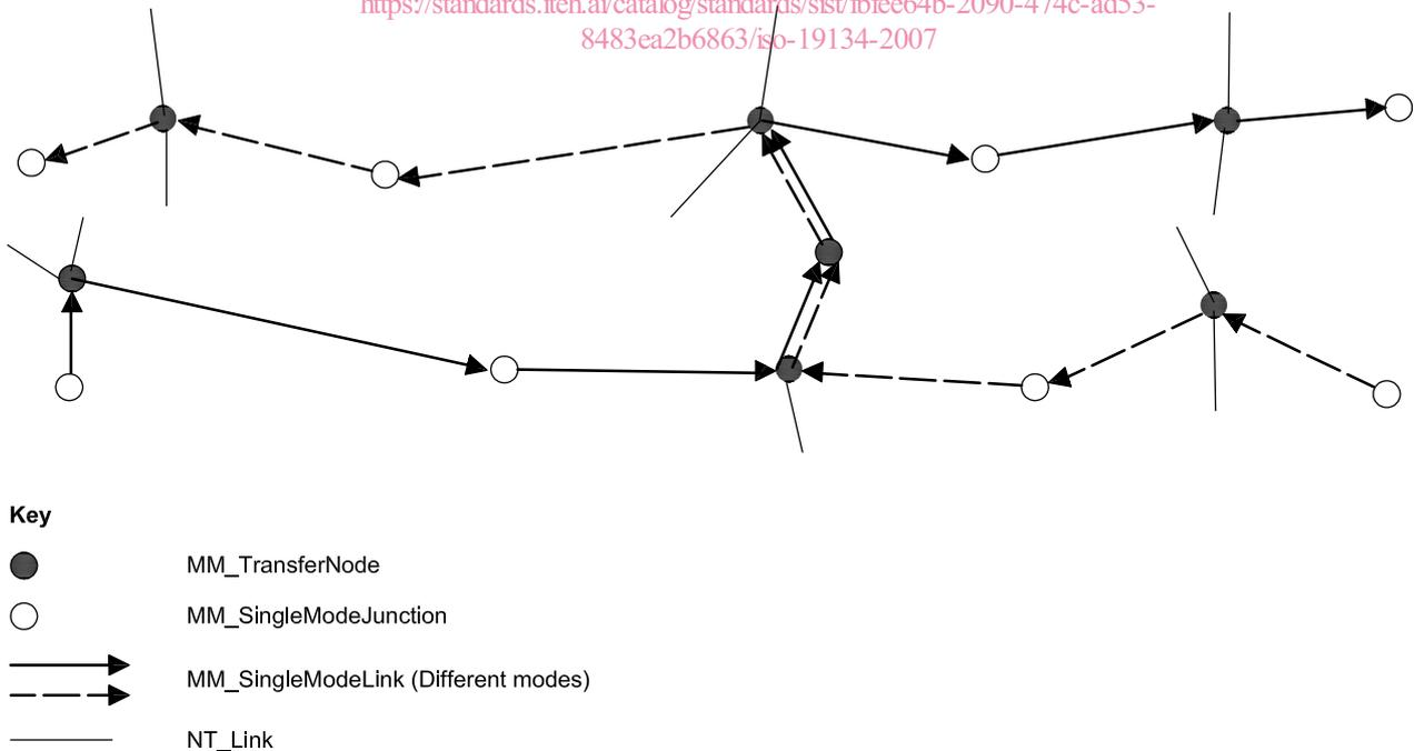
Figure 3 — NT\_SingleModeLinks and NT\_SingleModeJunctions in the MM\_MultimodalNetwork
