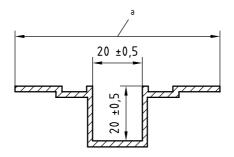
a Dimension adapted to the solder bath or the wetting balance
