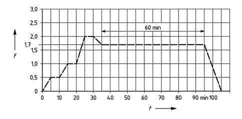
*f* is the factor to be applied to PN during the testNOTE The pressure changes need not be at a linear rate.
