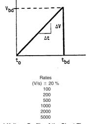
FIG. 1 Voltage Profile of the Short-Time Test
