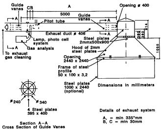
FIG. 1 Canopy Hood and Exhaust Duct
