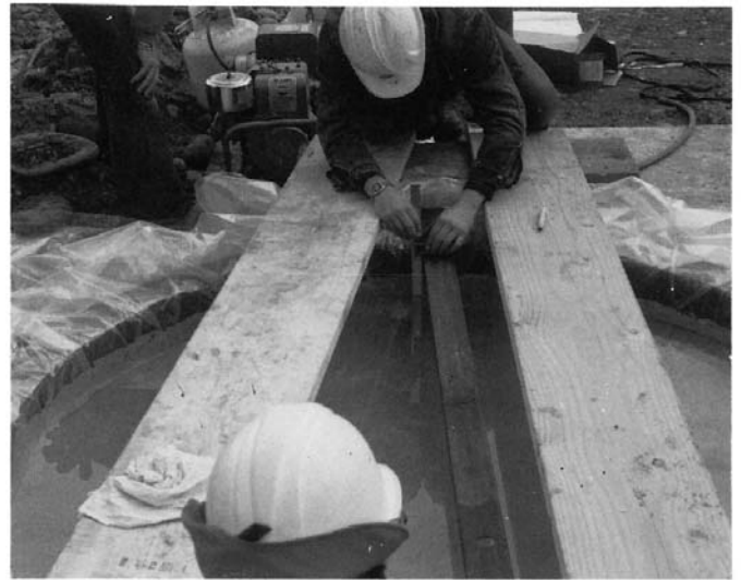
FIG. 3 Measuring the Water-Level Reference with a Carpenter's Square
