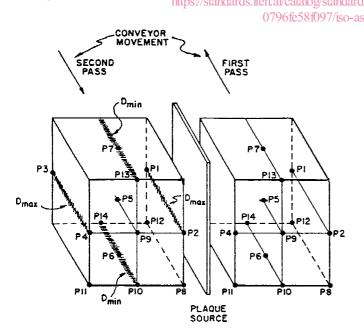
Note—Two passes of a rectangular package, one on each side of a stationary gamma-ray plaque source. The probable regions of maximum and minimum absorbed dose after the second pass are indicated by hatching. The recommended locations for dosimeters during irradiator characterization are indicated by the Ps.
