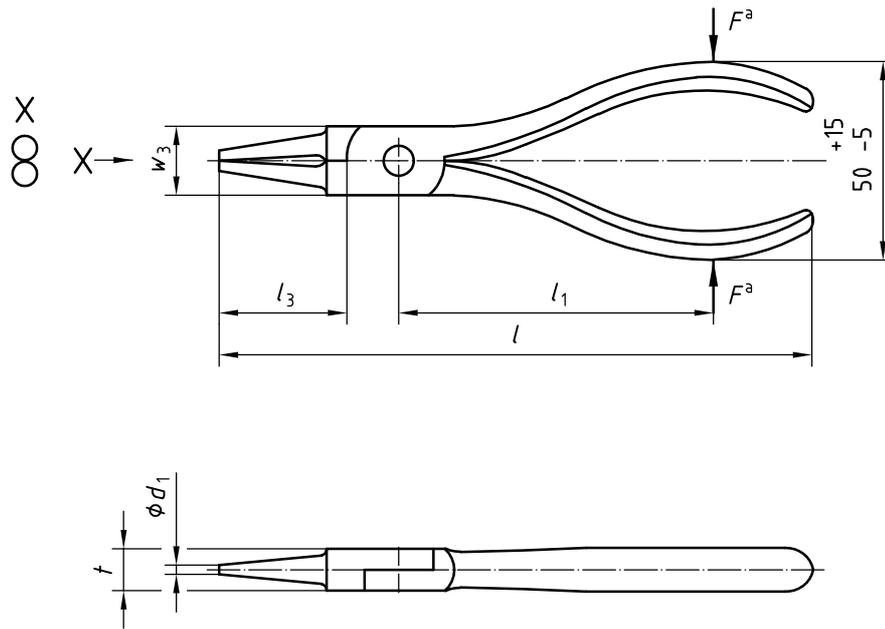
a  $F$  = Load applied in load test.
